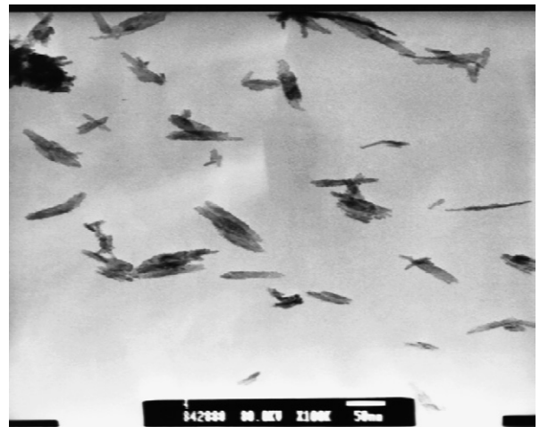
Fig. 3. TEM image of nanoparticles (approximately 90 nm in length and 30 nm in width).
